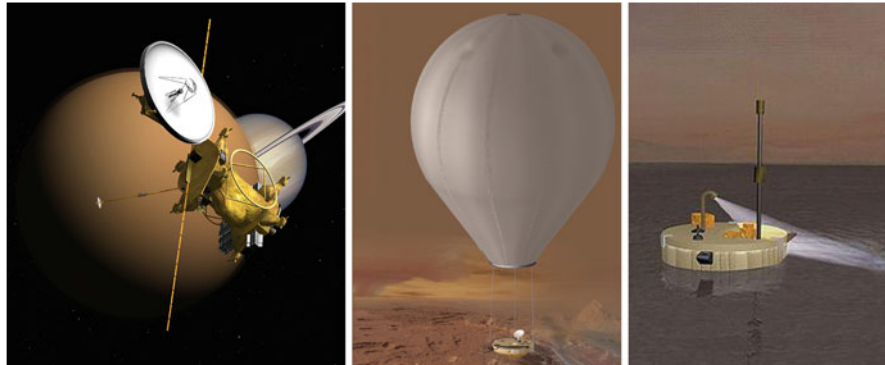
Figure 15. The TSSM basic concept. The orbiter ( left ), the balloon ( center ), and the lake lander ( right ) (Reh et al., 2008).
