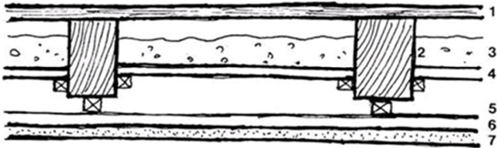
Sections of a traditional floor and a traditional roof in continental Greece and the islands of the Northern Aegean. In both cases earth in the structure's interior works as insulation. Floor: 1. Upper surface 2. Beams 3. Earth 4. Boards supporting the earth 5. Little beams 6-7 different layers of lime mortar
