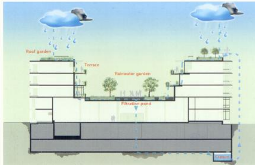
19.8 Rainwater harvesting diagram.
