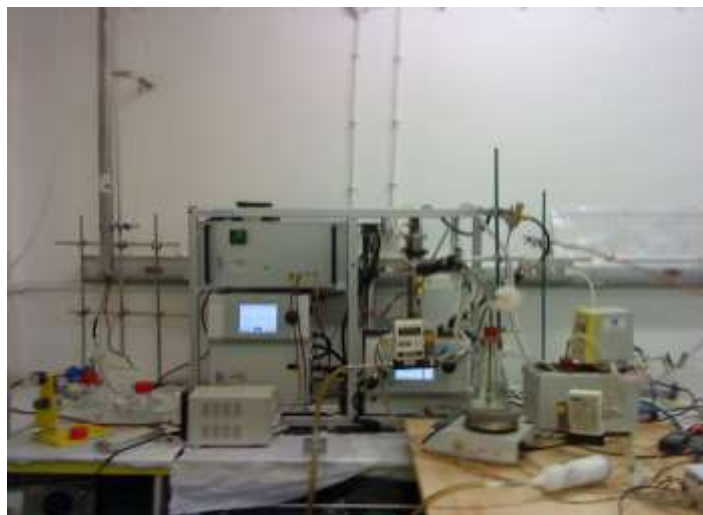
Picture A1: The HTDMA system during calibration and testing. The main components of the system (DMAs, CPC) are located in the metal frame (center of the photograph). The atomizer that was used is also visible on the left.
