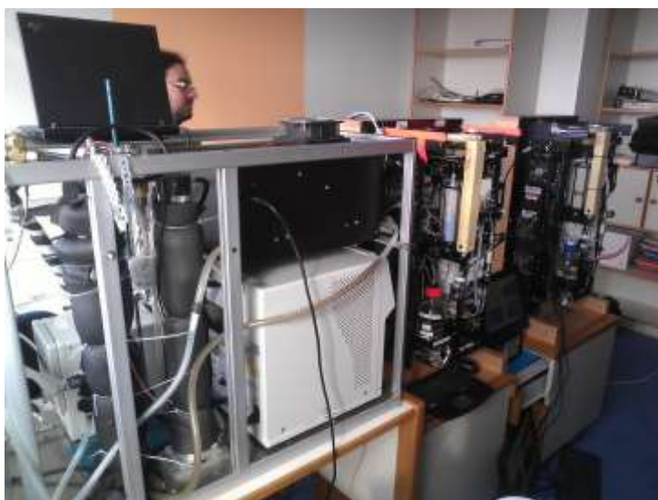
Picture A2: The HTDMA system during campaign measurements. The HTDMA system (on the left) was combined with one Cloud Condensation Nuclei (CCN) counter (located in the center) in order to provide fine and ultrafine particles hygroscopicity measurements in sub/super- saturation conditions
